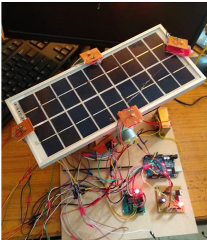
Fig -5: Hardware kit of Solar tracking System
