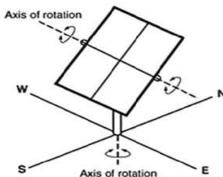
Fig - 4: Two axis Tracking system
